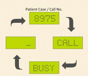
The Door Display Module is located next to the door frame at the entrance to the examination room. Its display alternates the called patient / case no. with a message saying 'CALL'. After the patient is in the room, the examining Doctor may operate the Room Unit keypad to change this message to BUSY' to forestall inadvertent entry by others while the patient is undergoing examination.
